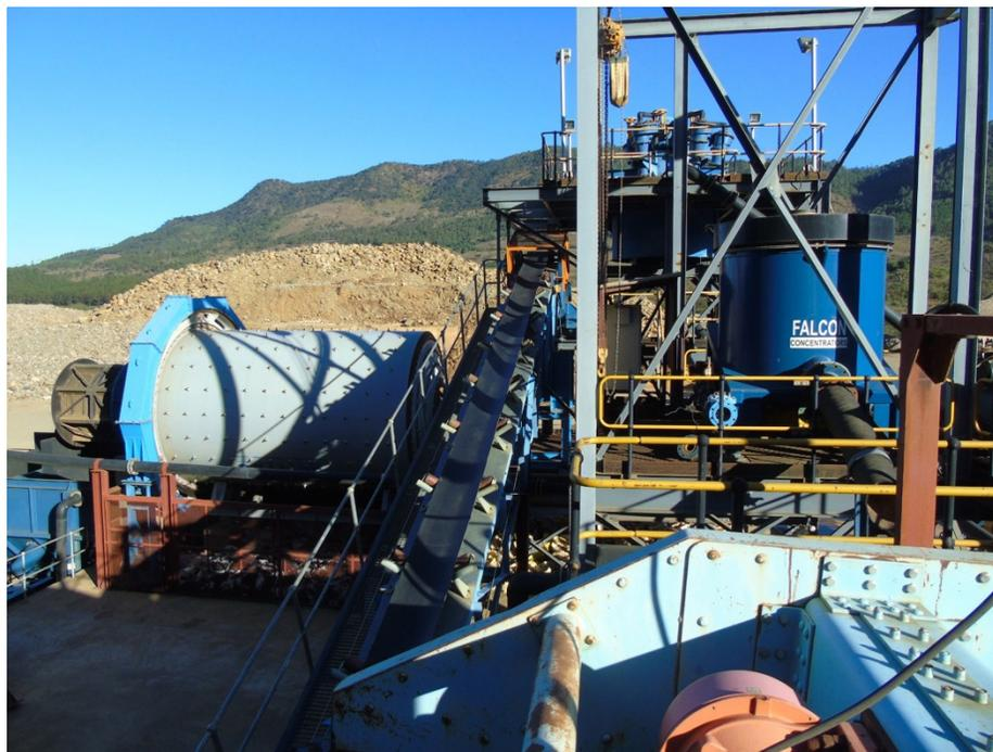
**Image 1.** Manica Gold Project – Existing Mill and Grinding Circuit
